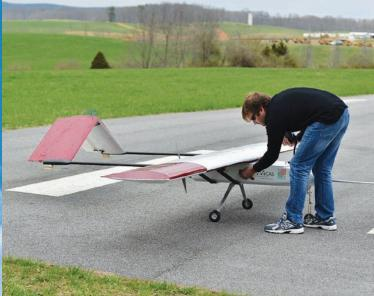
John Coggin removes the safety key from ESPAARO prior to flight.
