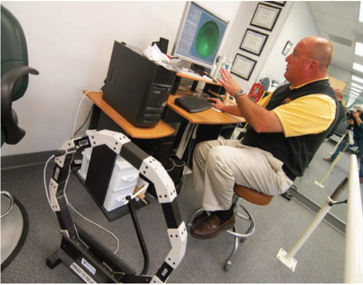
Doug Call looks at the scan created by the OMEGA Tracer System. The computer image is used to make, in this case, a new leg.
