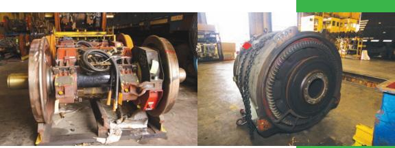
**Traction motor wheel assembly**
