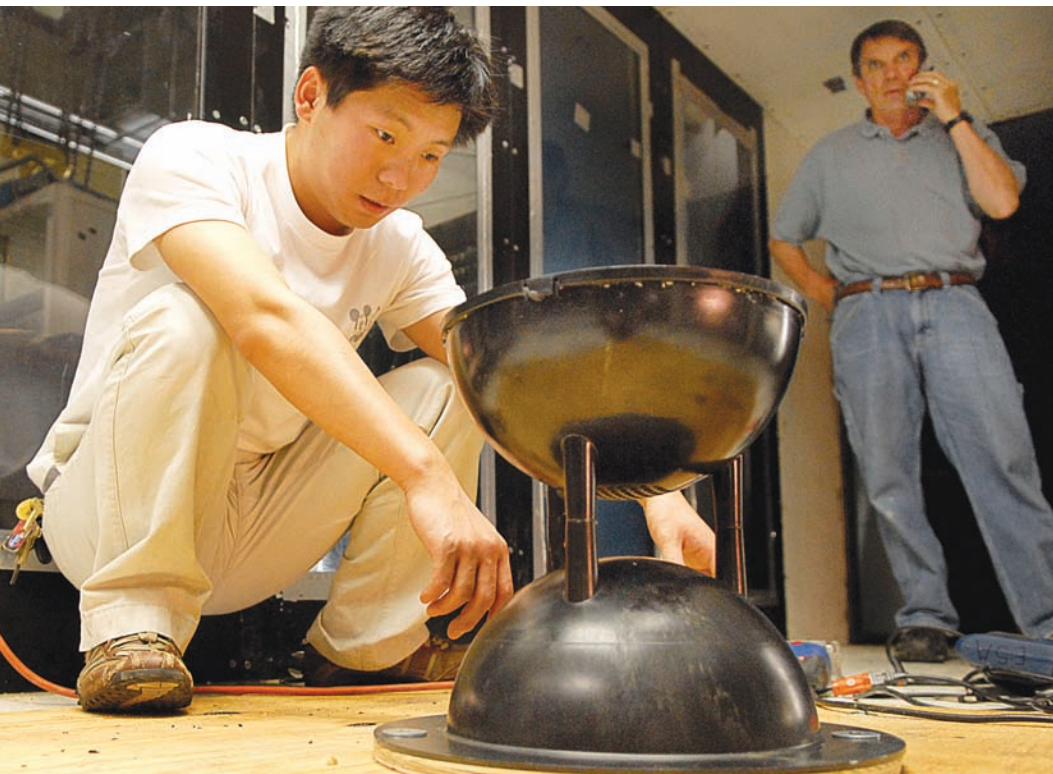
Acrylife's Pat Johnson watches grad student Yihong Yang install the prototype roof vent in the Virginia Tech stability wind tunnel.
