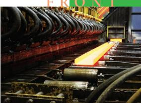
Heat-treated steel ready to be cooled.
