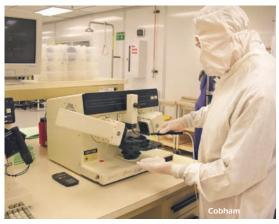
Terry Reed checks the thickness of a film on a wafer of MMIC chips.
