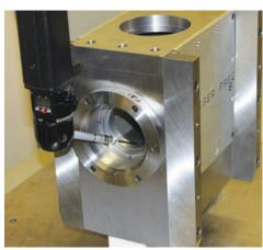
In the inspection room highlighting the use of the CMM machine to accurately determine a part's dimensional tolerances
