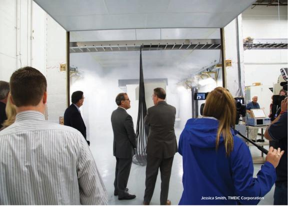
Guests look on as high humidity is simulated inside the TMEIC Photovoltaic Inverter Test Lab, one of many environmental conditions the \$1.5 million purpose-built facility is capable of generating.
