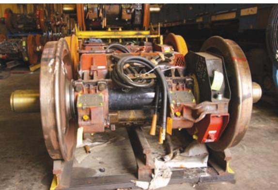
**Traction motor wheel assembly**
