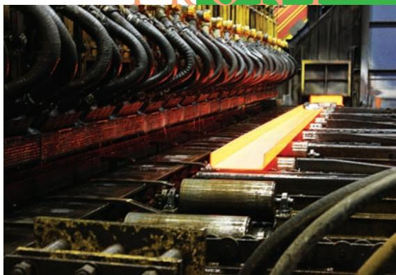
Heat-treated steel ready to be cooled.
