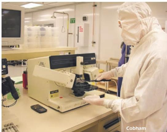
Terry Reed checks the thickness of a film on a wafer of MMIC chips.
