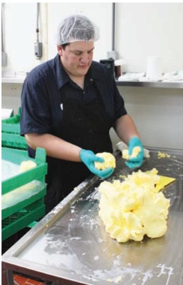
**Butter being packed into molds.**
