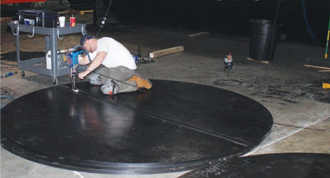
An AppTech plastic welder at work; the long line from the spool is plastic feeding the tool.
