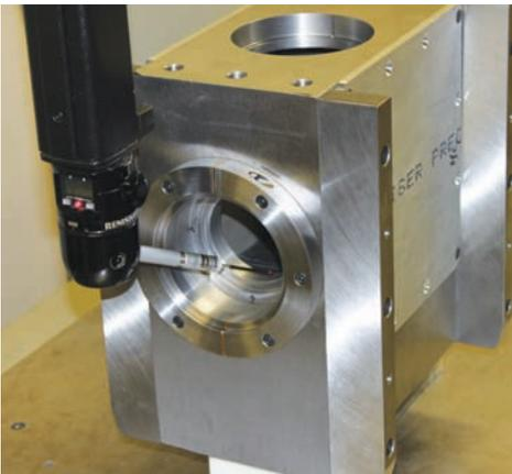
**In the inspection room highlighting the use of the CMM machine to accurately determine a part's dimensional tolerances**
