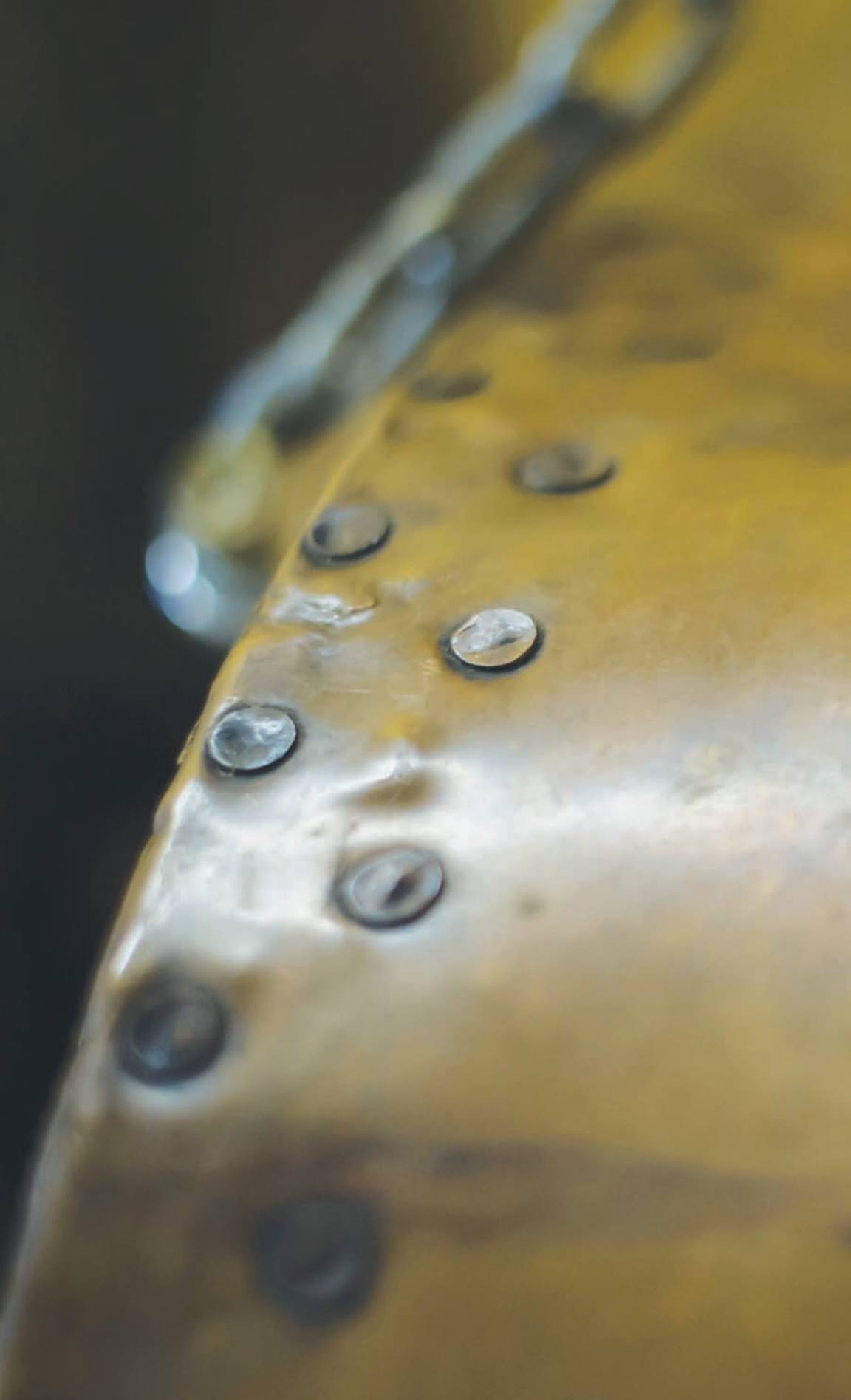
Original copper nails, straightened and reused in a renovated copper submarine still
